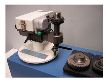
The measuring system allows the control of gear with pitch diameter between 20 and 200 mm and allow a precise adjustment of the ball alignment with the gear under exam that can be moved vertically in a field of 50 mm.
